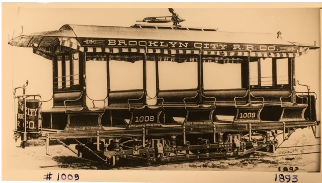
Car #1009 from the first usage of the 1000-series, an open horsecar made by Lewis & Fowler in 1885-86, operated by Brooklyn City Railroad, retired in 1898
