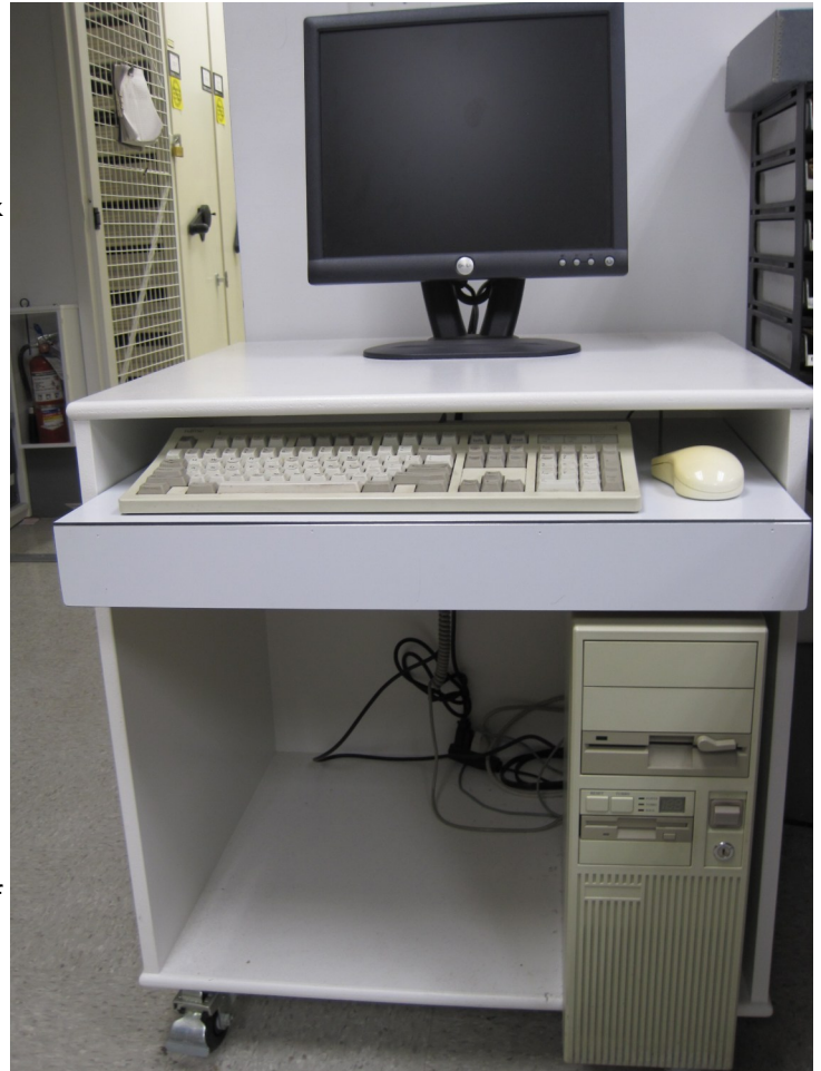
This digital archival work station employs an old CPU with floppy drives. The work station will be used in a later phase of the ERM program to read files from disks uncovered during the survey.
